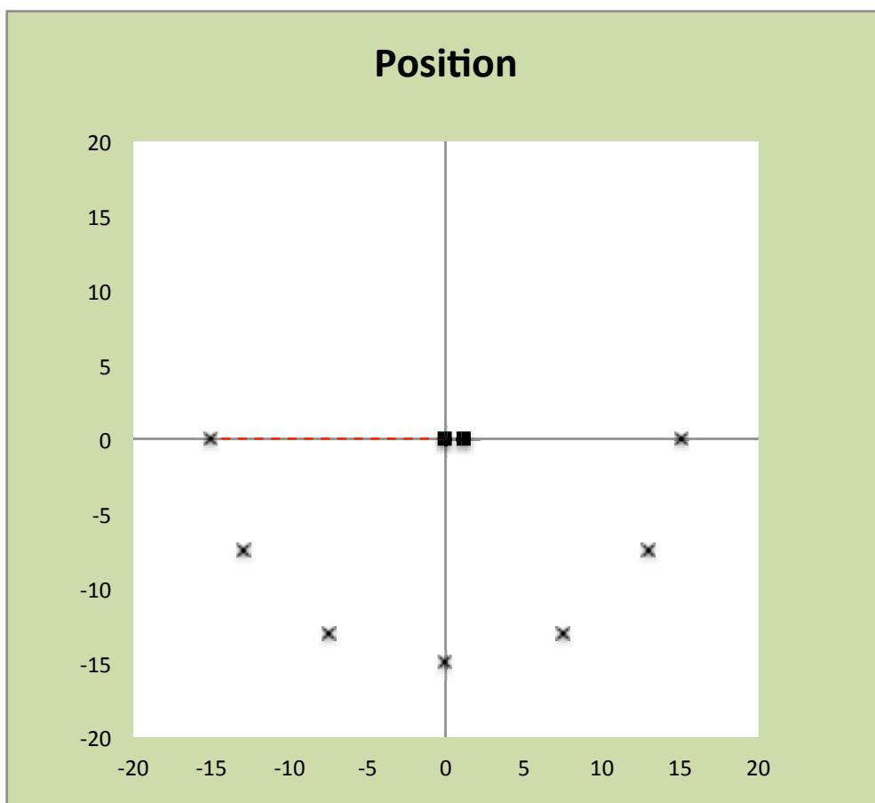
Both speakers can be seen as well as the 7 microphones positioned in a half circle at a distance of 15 m. The red dotted line indicates the microphone arc and always ends at the last microphone (No. 7).
