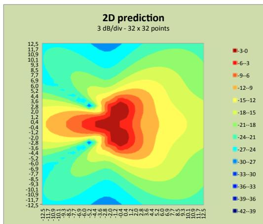
In some speaker setups e.g. a physical horizontal array with omni sources, a focal point appears behind the array that contains more energy in comparison to the front of the array. With full-space normalization this would lead to attenuated polar plots in front of the array and consequently incorrect -6 dB values.
