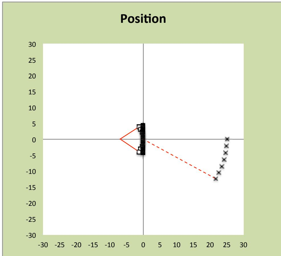
The 10 speakers and the 70° virtual arc angle can be seen. The 7 microphones are distributed equidistant over a 30° angle at 25 meters (global radius).
