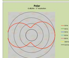
Both SPL and polar plots clearly show the focal node with greater output behind the array.
