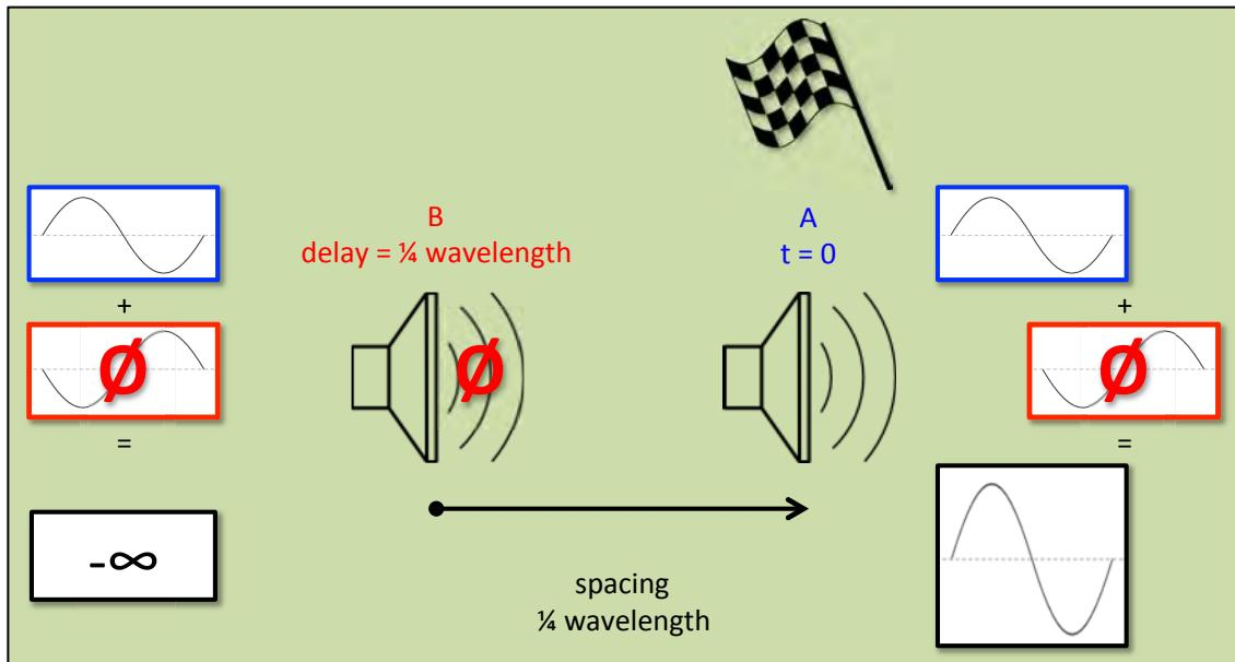
The illustration above shows the principle of the gradient configuration.
