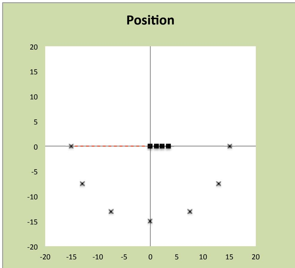
Four speakers can be seen as well as the 7 microphones positioned in a half circle at a distance of 15 m. The red dotted line indicates the microphone arc and always ends at the last microphone.
