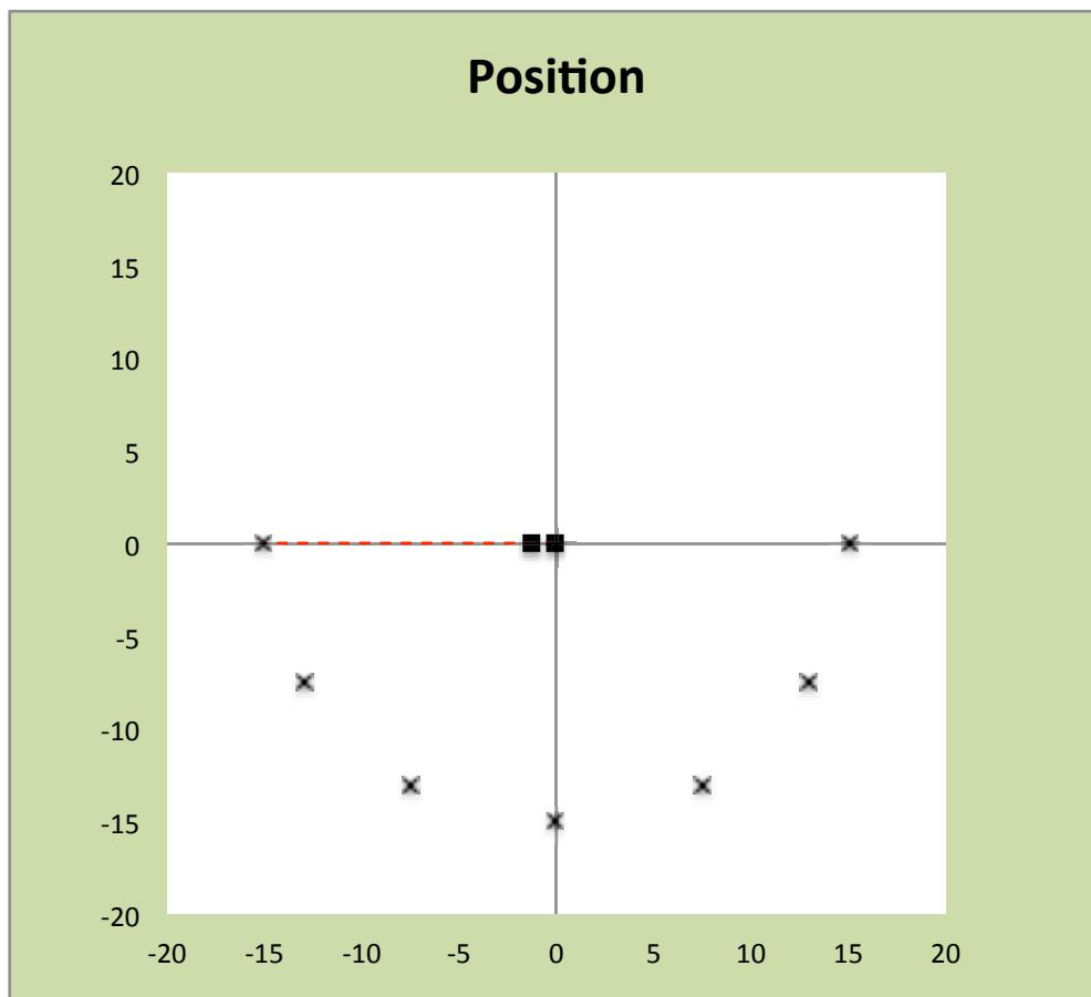
Both speakers can be seen as well as the 7 microphones positioned in a half circle at a distance of 15 m. The red dotted line indicates the microphone arc and always ends at the last microphone.
