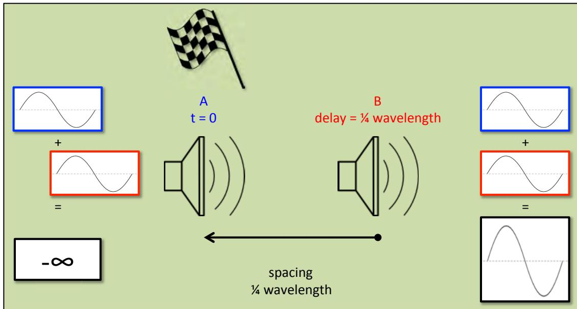
The illustration above shows the principle of end-fired configurations.
